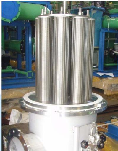
It is an automatic strainer that filters by installing a number of candle-shaped filter screens in a certain arrangement, and discharges impurities by differential pressure.
